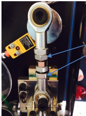
Figure 27. To adjust the length of the connection pole, release either of the two nuts located on the connection pole. Turning the nuts clockwise will cause the connection pole to lengthen. Turning the nuts counterclockwise will cause the connection pole to shorten.
