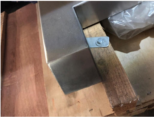
Figure 5. Bolts locking FRM-1120C to crate.
